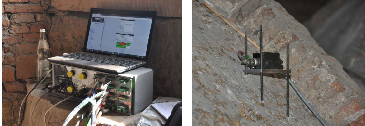
a) Data acquisition central, computer equipment and b) force balanced accelerometer
