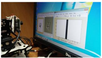
Fig. 11: Hardware setup for moving the DVS with a pan-tilt unit
