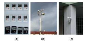
**Figure 1.** Instruments are measuring devices used for tests. (**a**) sensors of measurement (temperature and humidity); (**b**) meteorological station, to be placed in the building cover; (**c**) protective caps to prevent overheating of the sensor by direct radiation.
