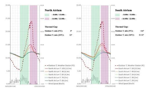
**Figure 3.** Comparative behavioral thermodynamic between the atriums. Note that the timetable of the morning and evening occupations of the building is indicated in green and purple respectively.
