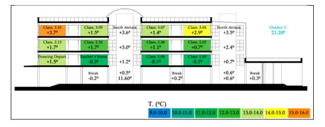
**Figure 4.** Thermal gaps correlation between classrooms and transitional spaces at 16:00 h (6 January 2019).
