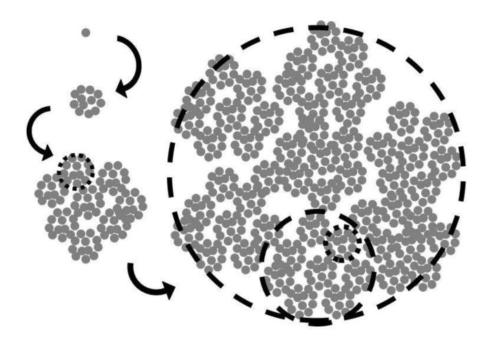
*Figure 2: Two examples of Cluster models with 3 shells of random-packed spheres and 2 hierarchical levels (left), and with 2 shells of random-packed spheres and three hierarchical levels (right).*
