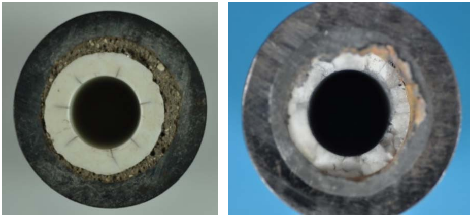
Figure 6. Cracks appearing in AT/M ceramic die a) during the wrapping process before ERS experiments, and b) after several processing cycles.
