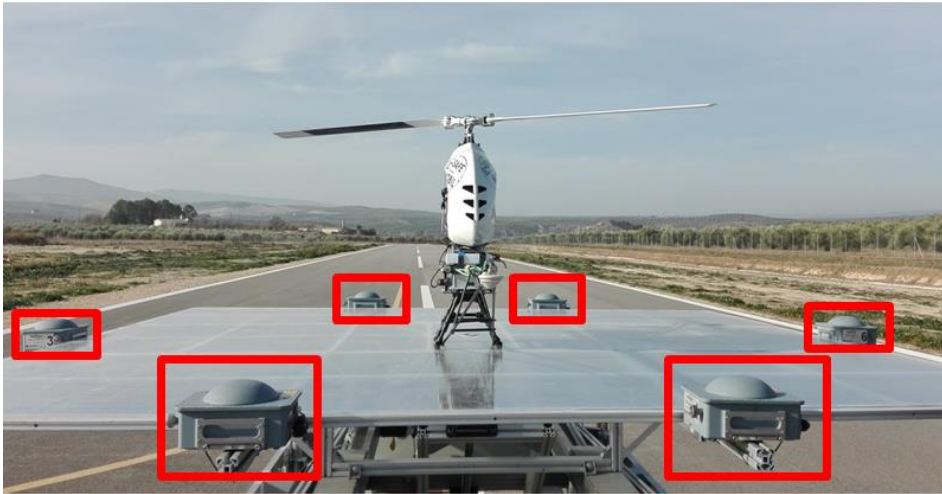
Figure 3-4: Ground segments units installed over a landing platform.
