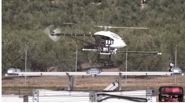
Figure 6-25: RPA with radio-beacon based navigator performing a landing.
