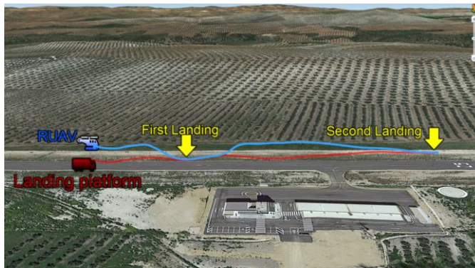
Figure 6-42: Rotary wing UAV trajectory landing on the moving platform using the tether in the straight trajectory test.
