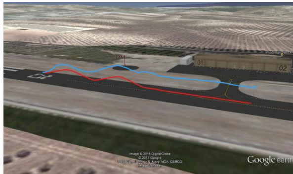
Figure 6-21: Rotary wing UAV trajectory (blue) landing on the moving platform (red)
