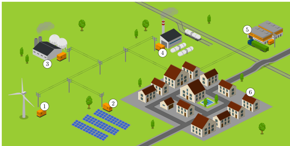
Figure 1. A MG (microgrid) considered in the problem, consisting of (1) a wind turbine, (2) photo-voltaic panels, (3) a microturbine, (4) a diesel engine, (5) an ESS (energy storage system), and (6) the demand.
