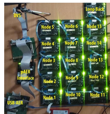
Fig. 1: Example setup of seventeen Spartan6 PCBs communicating through bidirectional LVDS SATA orthogonal links, plus a DVS camera and USB-AER board communicating through parallel AER buses with one of the Spartan6 PCBs.
