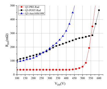
Figure 8. Multi-pulse test for GaN MISHEMT Q3 subjected to drain and gate voltage stress during irradiation.
