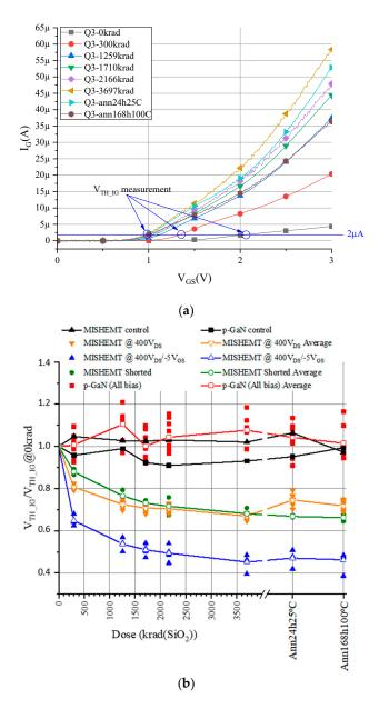
**Figure 4.** (a) Gate Schottky diode characteristics  $I_{GS}-V_{GS}$  (input characteristic) for  $V_{DS} = 0.1$  V. (b) Normalized threshold voltage measured for a gate current of 2  $\mu$ A.
