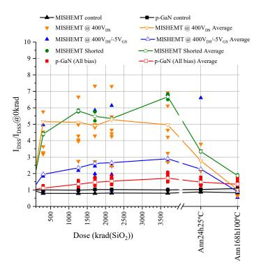
**Figure 5.** Normalized drain-to-source leakage current when applying a positive gate voltage of 500 V at the drain with 0 V at the gate.
