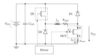
Figure 1. Circuit diagram used to measure R<sub>ON dyn</sub>.
