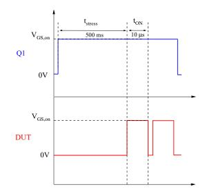
Figure A1. Gate voltage sequence for the double-pulse test.
