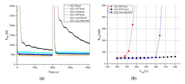
**Figure 10.** R<sub>ON\_dyn</sub> measurement for GaN MISHEMT Q22 subjected only to drain voltage during irradiation: (**a**) double-pulse measurement at 500 V, and (**b**) multi-pulse test measurement.
