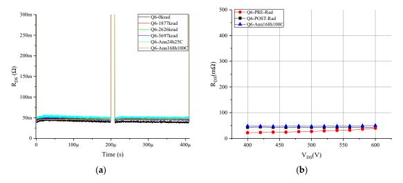
**Figure 9.** R<sub>ON\_dyn</sub> measurement for GaN MISHEMT Q6 subjected only to drain voltage during irradiation: (**a**) double-pulse measurement at 500 V, and (**b**) multi-pulse test measurement.
