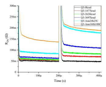
**Figure 7.** R<sub>ON\_dyn</sub> double-pulse measurements at 500 V for GaN MISHEMT Q3 subjected to drain and gate voltage during irradiation.
