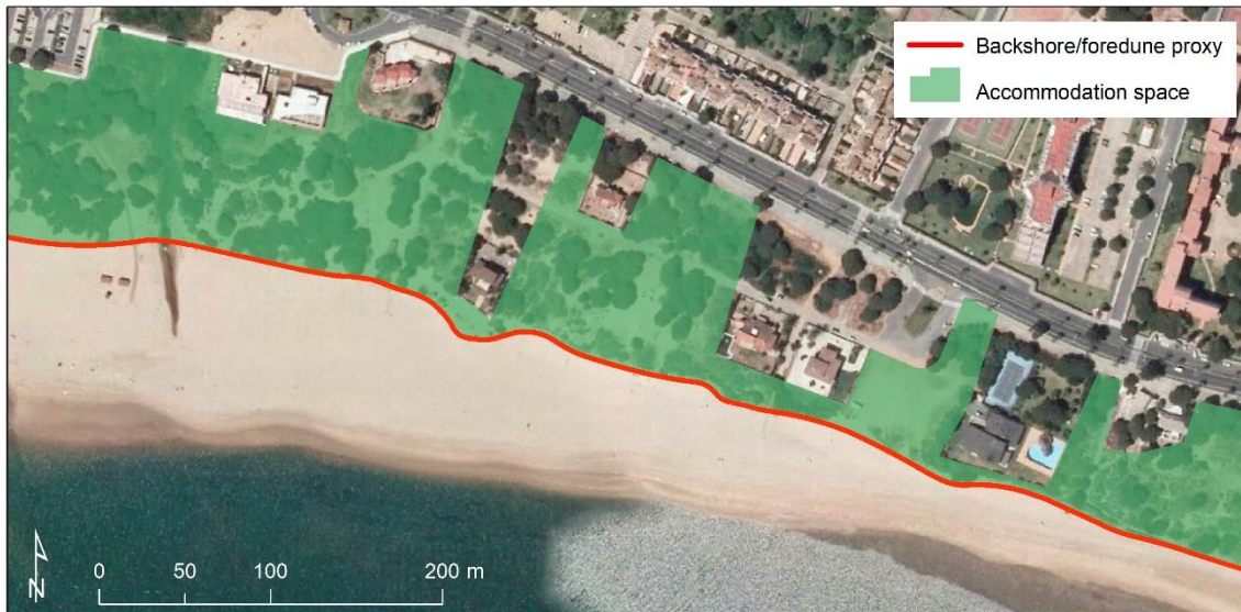
Figure 4. Photo-interpretation and digitisation of accommodation space based on the backshore/foredune proxy of the 2013 shoreline.
