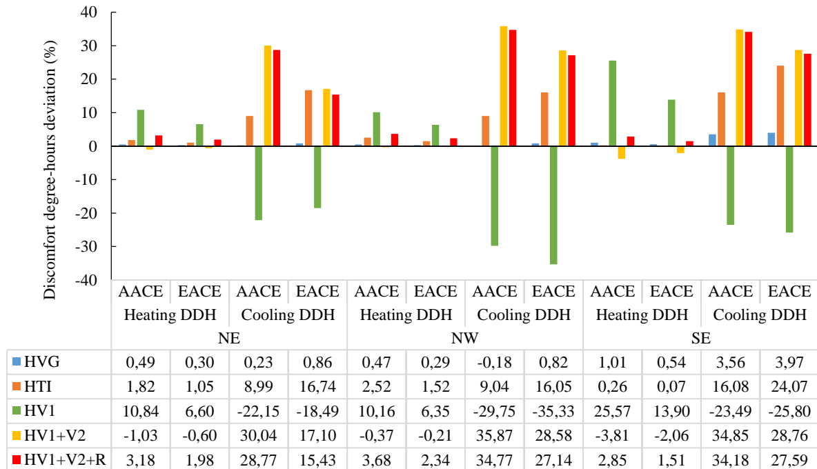
Fig. 10. Discomfort degree-hours deviation (%) of the hypotheses tested on the Base Case , according to AACE [46] and EACE [47].
