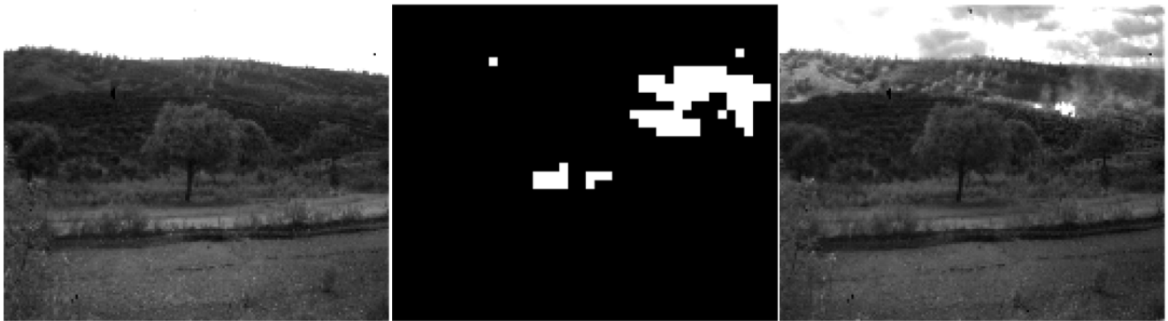
Figure 6 – Initial background (left), foreground segmentation (center) and image sent via radio by Wi-FLIP (right) during one of the field tests carried out.
