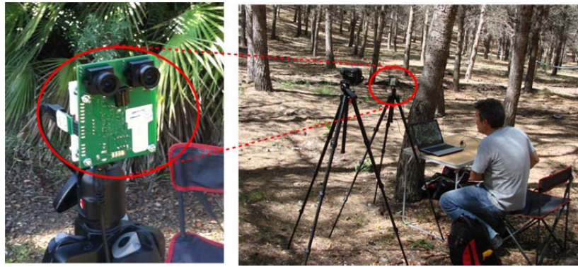
Figure 5 – Silicam IGO platform capturing images for on-site smoke detection.
