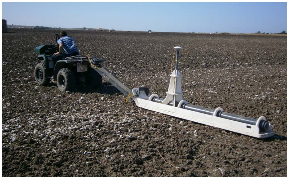
Figure 2.3 Dualem 21-S sensor working in the field.
