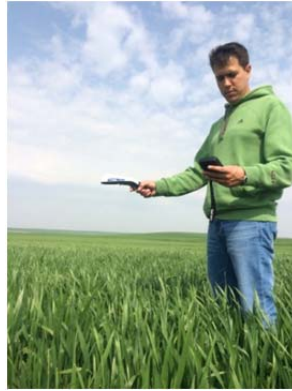
Figure 3.1 Hand-held NDVI sampling system in the experimental field.
