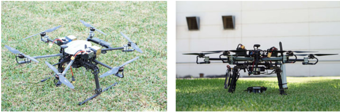
FIGURE 3 Aerial platform developed for the Challenge. Left, airframe without the mission electronics and the pickup mechanism. Right, fully equipped hexacopter [Color figure can be viewed at wileyonlinelibrary.com ]
