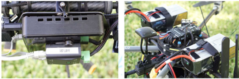
FIGURE 4 Front view (left) and side view (right) of the aerial platform with all the sensors and electronic devices on board. The spatial distribution of the equipment is indicated [Color figure can be viewed at wileyonlinelibrary.com ]
