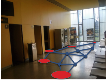
Fig. 2 The space is discretized by learning a topological map from people tracks obtained with the robot sensors (in blue). Some of the nodes are identified during the learning phase as goals (in red).
