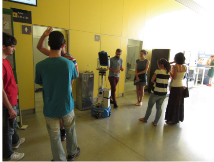
Fig. 1 The telepresence robot is located in a meeting area, and the task consists of approaching people that go to typical interaction points (like coffee machines). These points of interest are learnt previously from data.
