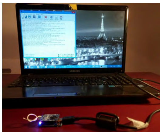
FIGURE 9. The receiver module receiving the location data of the radio beacon and sending them to a laptop.
