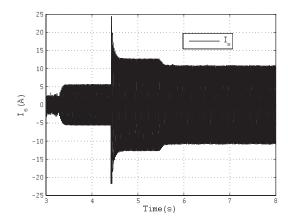
Fig. 18. Evolution in time of grid current.
