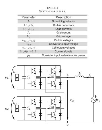
Fig. 1. Two-cell single-phase CHB power converter.
