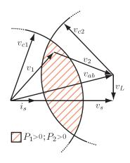
Fig. 4. Stable control area when  $v_{c1} \le v_{ab}$  and  $v_{c2} \le v_{ab}$ .
