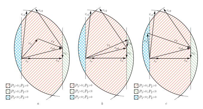
Fig. 8. Stable control area when  $v_{c1} > v_{ab}$  and  $v_{c2} > v_{ab}$ . From left to right: Possible solution with: a)  $P_1 > 0$  and  $P_2 > 0$ . b)  $P_1 > 0$  and  $P_2 < 0$ . c)  $P_1 < 0$  and  $P_2 > 0$ .
