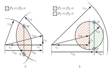
Fig. 11. Set of possible solutions for a particular active power distribution. From left to right: a)  $v_{c1} \le v_{ab}$  and  $v_{c2} \le v_{ab}$ . b)  $v_{c1} > v_{ab}$  and  $v_{c2} \le v_{ab}$ .
