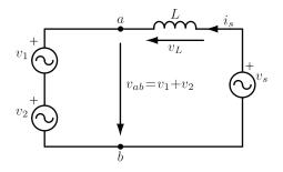
Fig. 2. 2C-CHB equivalent circuit.
