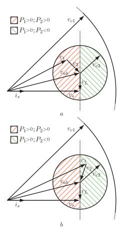
Fig. 6. Stable control area when  $v_{c1} > v_{ab}$  and  $v_{c2} \le v_{ab}$ . From top to bottom: Possible solution with: a)  $P_1 > 0$  and  $P_2 > 0$ . b)  $P_1 > 0$  and  $P_2 < 0$ .
