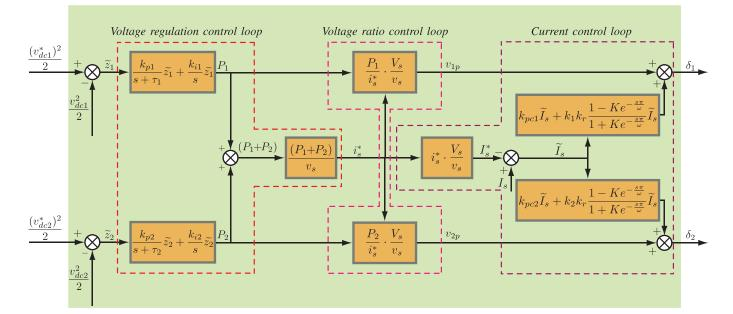
Fig. 10. Block diagram of the system controller.
