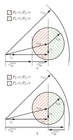
Fig. 7. Maximum and minimum active power limits when  $v_{c1} > v_{ab}$  and  $v_{c2} \le v_{ab}$ .
