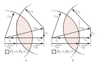
Fig. 5. Maximum and minimum active power limits when  $v_{c1} \le v_{ab}$  and  $v_{c2} \le v_{ab}$ .
