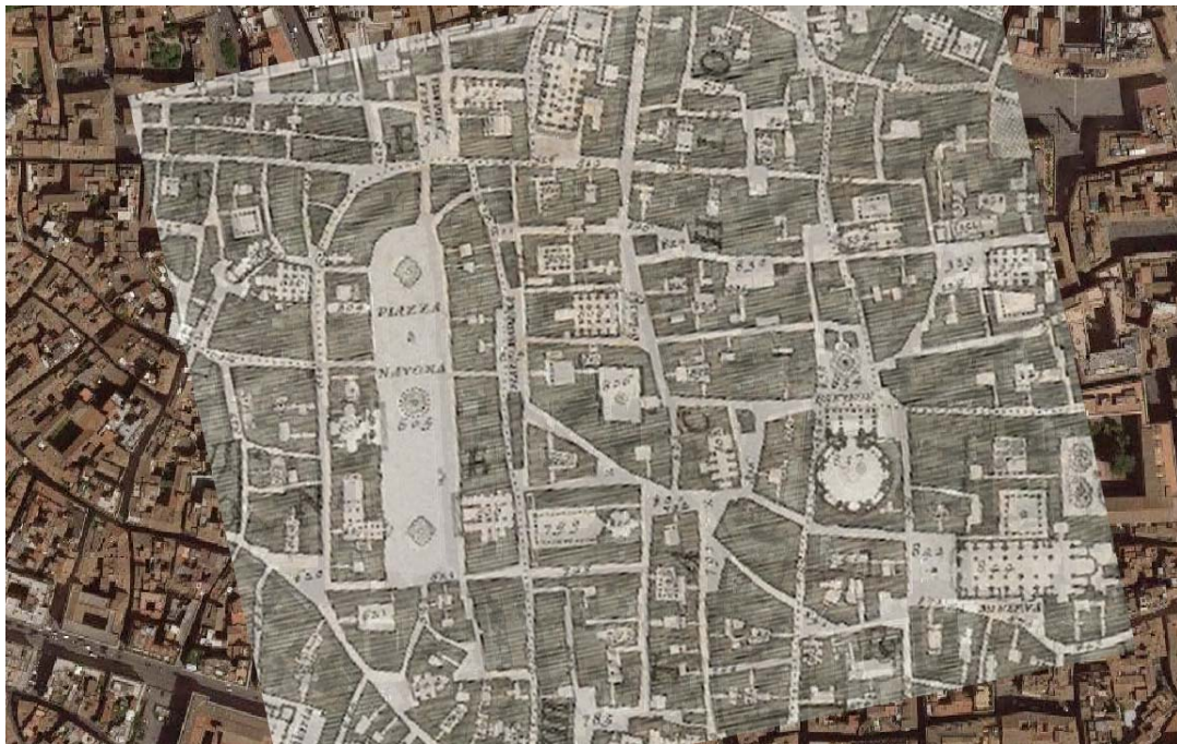
Figure 3. Area Piazza Navona-Pantheon (Rome, Italy). Overlay of the Nolli plan (1748) and the current plan of the city of Rome (source: Google Maps). The millimeter precision of the nineteenth-century plan shows how scientific methodology is introduced in cartography.
