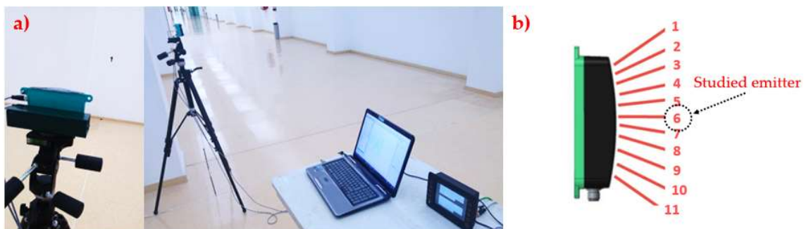
Figure 3. (a) Sensor arrangement for accuracy laboratory test, (b) tested LED emitters.
