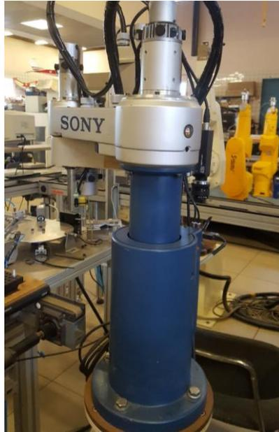
Figura 2-5. Robot Sony SCARA.
