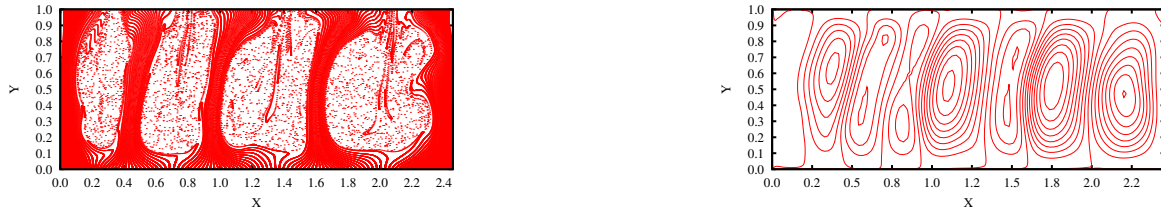
Figure 11. Particle distribution (left) and stream function (right) for L = 4 * L_{\text{linear}} , C = 10 , Re_E = 1.0 and T = 400 with FE-PIC. at time t = 6.0 . Up to seven rolls can be discerned. The boundary conditions are no-slip at the right and left sides.
