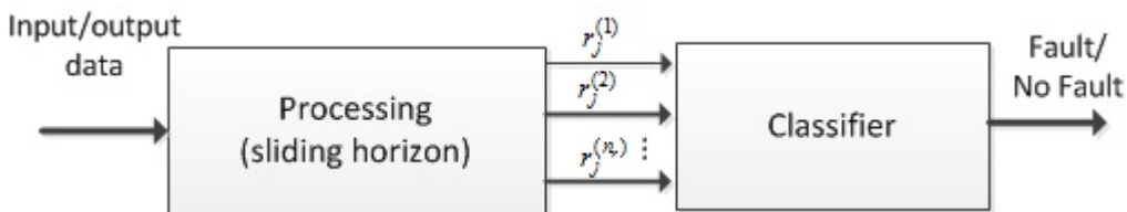
Figure 5.1: Fault detector scheme on line
