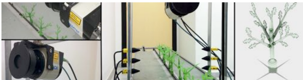
Figure 1. Details of the sensors on the laboratory platform (LiDAR and IR light beam) for the detection and structure of the modular 3D plant (left).
