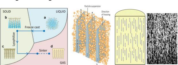
The frozen liquid dendrites are then sublimation, removed by and pore is generated elongated instead. Finally, the sample green must be under sintered an appropriate atmosphere.
