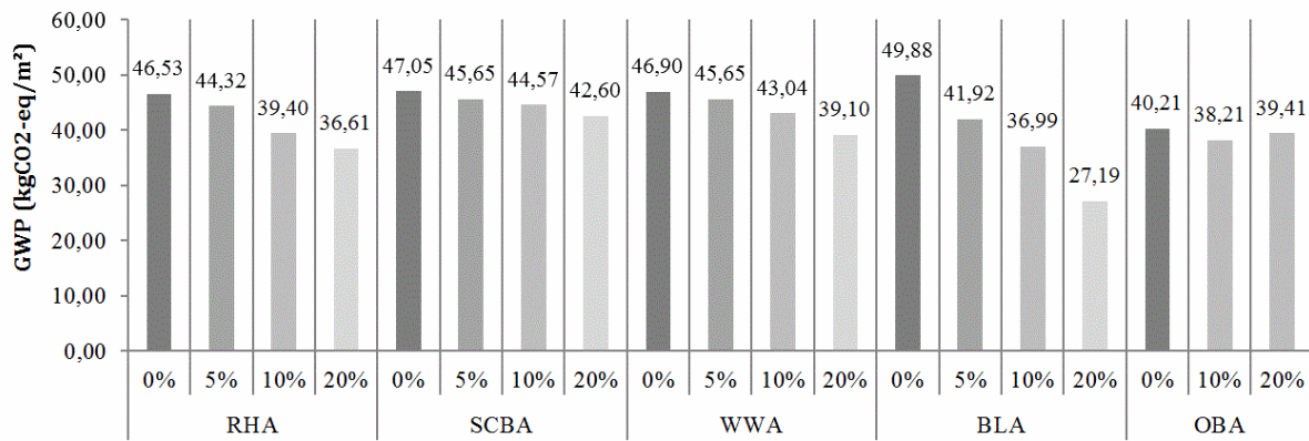
Figure 2 Global Warming Potential of biomass ash-cement compounds ( \text{kgCO}_2\text{-eq/m}^2 ) for different cement replacement percentage (from 0 to 20%) (González-Kunz R. , Pineda, Bras, & Morillas, 2017)
