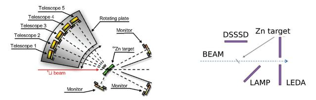
FIGURE 1. Sketches of the experimental setups of the <sup>6.7</sup>Li+<sup>64</sup>Zn (on left) and <sup>6</sup>He+<sup>64</sup>Zn (on right) measurements.
