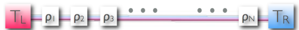
FIG. 2. The model is defined on lattice sites, each one characterized by an energy \rho_l . The dynamics is stochastic and proceeds via random collisions between nearest neighbors where part of the pair energy is dissipated to the environment and the rest is randomly redistributed within the pair. Such dynamics mimics at the mesoscopic level the evolution of a wide class of systems characterized by a nontrivial competition between diffusion and dissipation.
