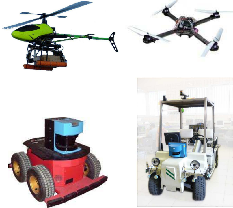
Figure 1.1: Multiple heterogeneous robots that may be part of a multi-robot system. Clockwise, starting from the top left: autonomous helicopter, aerial quadrotor, two ground autonomous vehicles.
