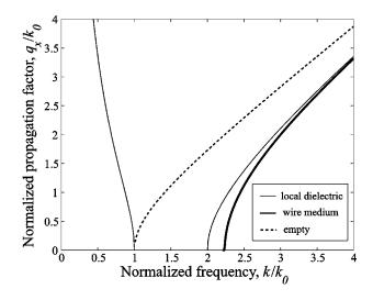
FIG. 2. Normalized propagation factors in a parallel-plate waveguide vs normalized frequency for different types of waveguide filling: Thin solid lines, uniaxial dielectric with a negative permittivity; thick solid line, wire medium; dashed line, empty waveguide. The wire medium and the uniaxial dielectric have the same  $k_0 = \pi/(2d)$ .
