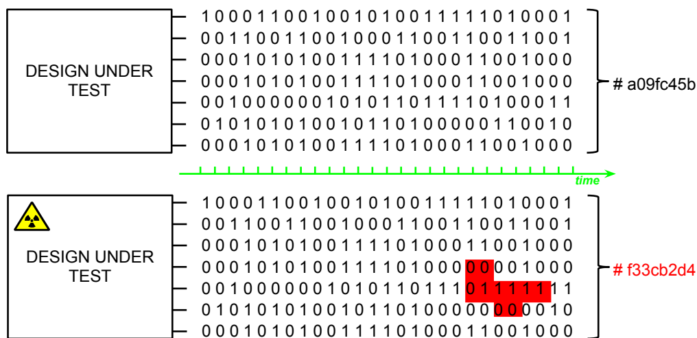
Figure 3.1: Figure on the top represents the normal data flow from the DUT output port and the associated hexadecimal signature or golden signature. Figure on the bottom represents the circuit operating under radiation, an erroneous data flow (the error pattern is shadowed) and the associated anomalous signature.
