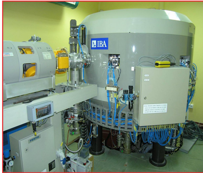
Figure 2.7: Cyclotron at the CNA. Protons were accelerated to 18 MeV for a first dynamic radiation experiment on a Xilinx CPLD [107].
