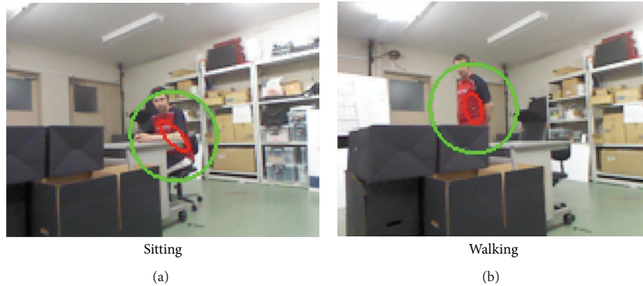
FIGURE 22: Sample robot system tracking and activity recognition results with partial occlusion cases for (a) sitting and (b) walking activities.
