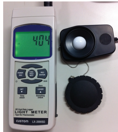
FIGURE 13: Illumination sensor: CUSTOM LX-2000SD light meter.
