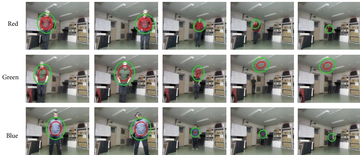
FIGURE 17: Fixed robot condition: tracking results with one-color representation.
