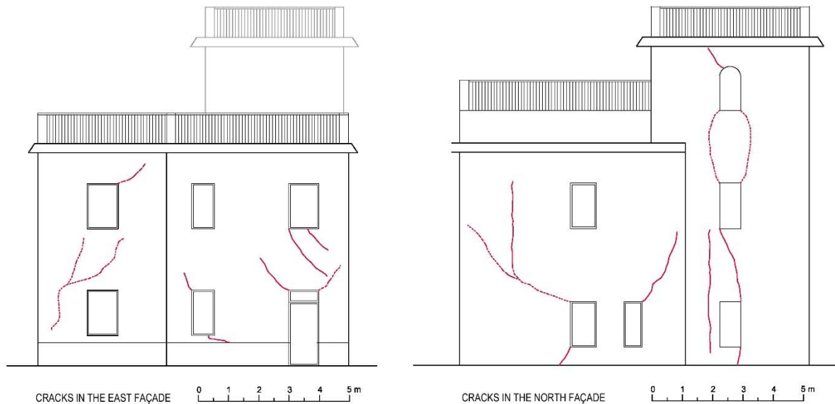
Figure 6. Maps of cracks in the east and north façades of the building.
