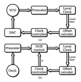
Fig. 1. Hardware clock models. (a) Computer model based on a VCO. (b) Proposed hardware clock model based on a fixed-frequency oscillator.
