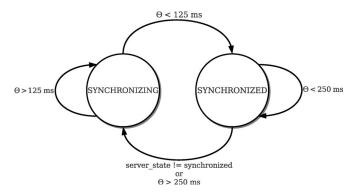
Fig. 3. States of the synchronization algorithm.
