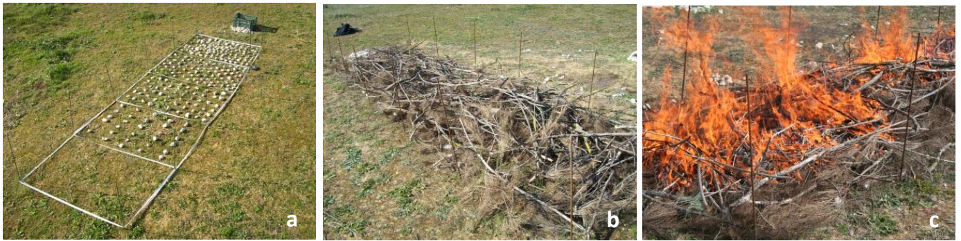
Figure 1. Some details of the experimental work: (a) soil plots with 0, 15, 30, 45 and 60% stone cover; (b) soil plot after addition of fuel; (c) soil plot during burning.
