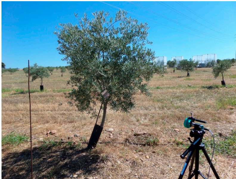
Figure 4. Positioning of the sensor for distance measurements in the field.
