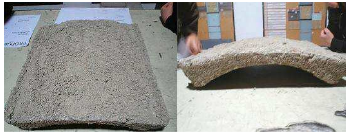
Fig. 8 “Small vault test with an existing mould Test 1 and 2”
