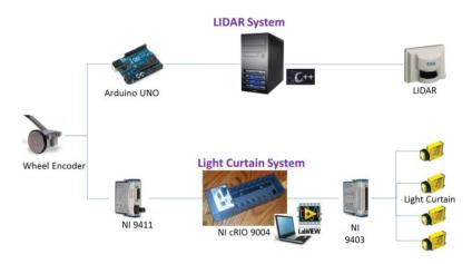
All of the necessary components for each of the aforementioned systems (LIDAR and light curtain, Figure 2) were recorded in a parallel fashion using the encoder value for future event synchronization and evaluation. In this way, two independent files were obtained from each optical sensor system and test.
