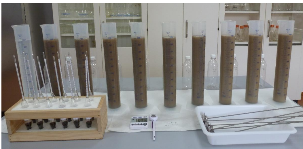
Figure 2.13 – Set of materials used for the measurement of soil texture by the Bouyoucos hydrometer method.
