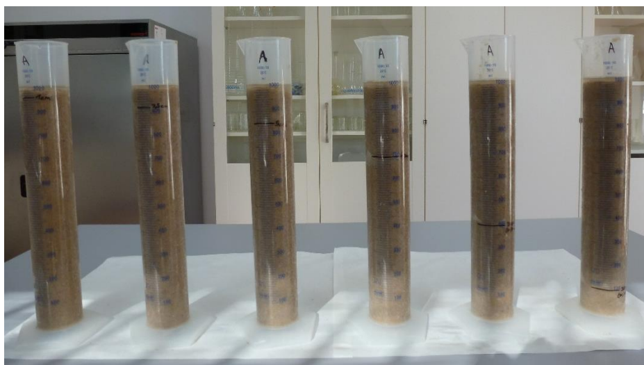
Figure 2.9 – Silica sand columns used for evaluating the impact of pressure on swelling properties of cross-linked potassium polyacrylate.
