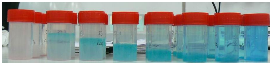
Figure 2.12 – Plastic bottles used in the potassium release curves experiment containing in this case \text{CuSO}_4 solutions.
