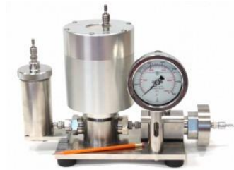
Figure 4.2-7: Avestin high pressure homogeniser
