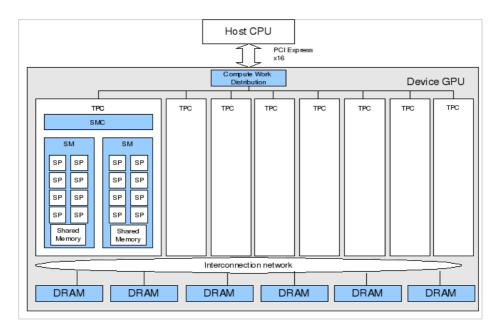
Fig. 1. Tesla Unified Architecture. TPC: Texture/processor cluster. SM: Streaming Multiprocessor, distributed among TPCs. SP: Streaming Processor.
