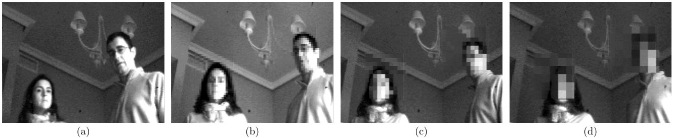
Figure 8. Real-time focal-plane reconfiguration conducted by the Viola–Jones frontal face detector. If faces are detected, the coordinates of the corresponding bounding rectangles are sent back to the test board for the vision sensor to reconfigure the image capture on-the-fly.
