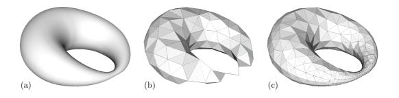
Figure 2: (a): original surface; (b): irreducible refinement; (c): stable refinement
