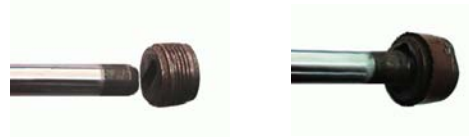
Figure 1: Pieces before and after the weld.
