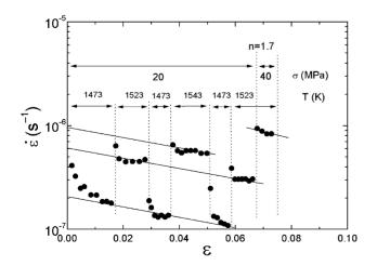
Fig. 3 Creep data plotted as  $\dot{\epsilon}$  vs.  $\epsilon$  for  $(La_{0.55}Sr_{0.45})_{0.99}Mn_{0.95}Ga_{0.05}O_3$ . The values of  $\sigma$ , T, and n are shown.
