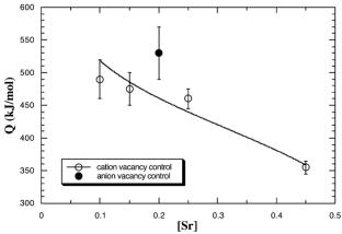
**Fig. 6** Variation of activation energy for creep as a function of [Sr] for undoped LSM. The filled point represent creep in the anion-vacancy-controlled region, whereas the open points represent cation-diffusion-controlled creep.<sup>2</sup> References for data for [Sr] < 0.45 are given in Table 1. The solid line is the weighted fit of the cation model<sup>2</sup> to the open points.
