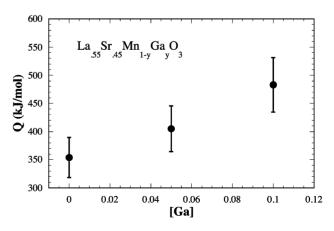
**Fig. 5** Variation of activation energy for creep as a function of [Ga]. Error bars reflect estimated uncertainties in strain rate, and temperature.
