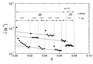
**Fig. 2** Creep data plotted as  $\dot{\varepsilon}$  vs.  $\varepsilon$  for undoped LSM,  $(La_{0.55}Sr_{0.45})_{0.99}MnO_3$ . Values of  $\sigma$ , *T*, and *n*, are shown.
