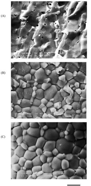
Fig. 1 Scanning electron photomicrographs of (A) fractured surface of LSM, (B) thermally etched surface of LSM for y = 0.05, and (C) thermally etched surface of LSM for y = 0.10.
