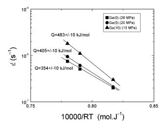
**Fig. 4** Arrhenius plots for undoped LSM and 5 and 10% Ga-doped LSM. Values of stresses for which plots were made are shown in the legend. Uncertainties shown are calculated from the least-square fits to the Arrhenius plots; they do not include uncertainties in temperatures and strain rates.
