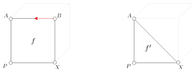
Fig. 3.27: The square face f is deformed into the triangular face f' , as a consequence of degenerating an edge which is incident to f .
