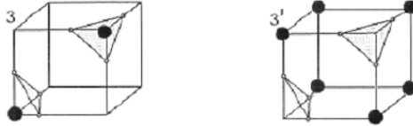
Fig. 2.23: On the left: the portion of surface corresponding to the Case 3 in Table 2.3. On the right: the portion of surface corresponding to the complementary configuration by choosing a neighborhood relation more restrictive between the unmarked vertices than between the marked vertices.
