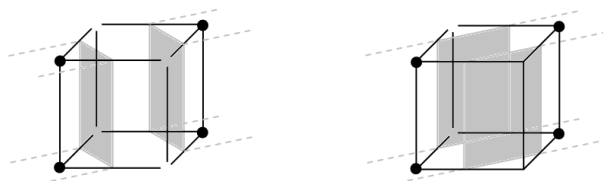
Fig. 2.25: The intersection points obtained by using linear interpolation give rise to both surfaces and it is not possible to take a decision on the interpretation of these types of situations.
