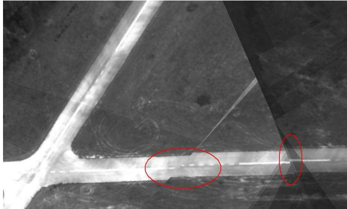
Figure 4.2: Piece of mosaic with global alignment errors (ellipses)
