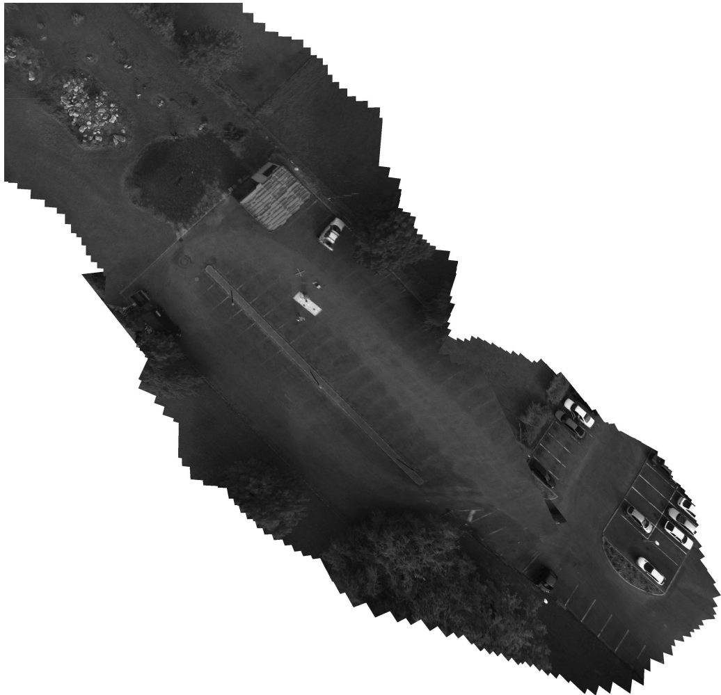
Figure 5.7: Mosaic of “le grand parking” at LAAS (Toulouse). KARMA was flying at 22 meter over the ground.
