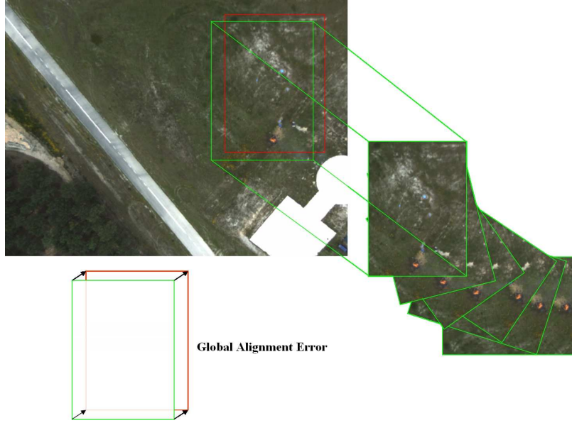
Figure 4.3: Global alignment errors due to accumulative misregistration. The red square denotes the correct position inside the mosaic. The green square marks the position computed by using local alignment
