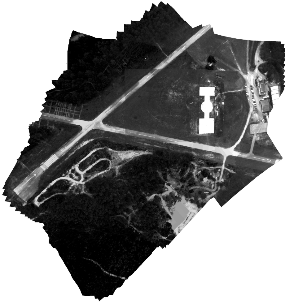
Figure 4.6: Lousa Airfield (Portugal). 3300 \times 3500 mosaic composed by more than 500 aerial images, with global alignment and color correction
