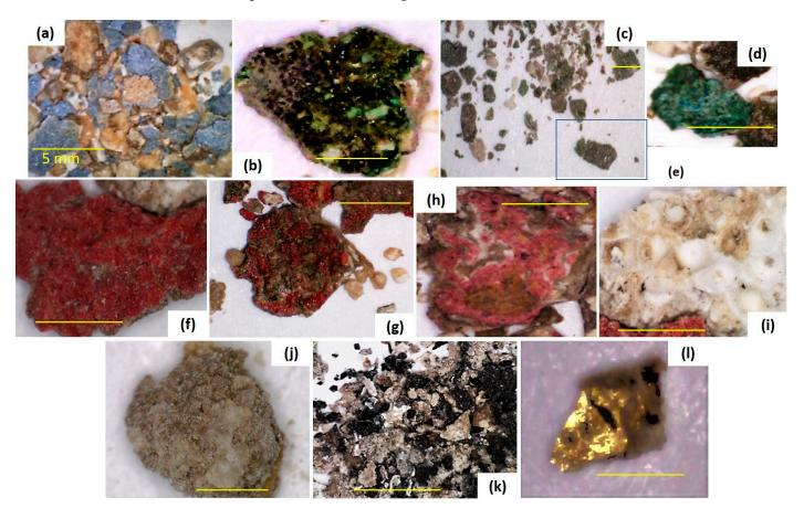
**Figure 3.** Micrographs corresponding to the different samples studied in this work: (**a**) blue sample 1; (**b**) green sample 10; (**c**) green sample 4; (**d**) green sample 5; (**e**) turquoise sample 9; (**f**) red sample 3; (**g**) red sample 2; (**h**) red sample 11; (**i**) support of the red sample 3; (**j**) yellow sample 6; (**k**) black sample 8; and (**l**) golden sample 7.
