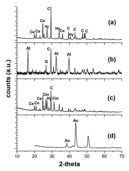
**Figure 5.** XRD diffractograms of the following samples: (a) blue 1; (b) green 10; (c) red 3; and (d) golden 7 [C = calcite, Hy = hydrocerussite, Ce = cerussite, At = atacamite, Q = quartz, Cin = cinnabar, and Au = gold].
