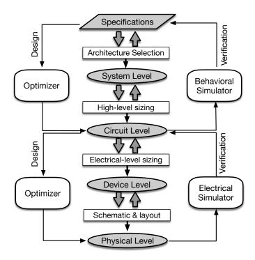
Fig. 1. Optimization-based top-down/bottom-up design process.
