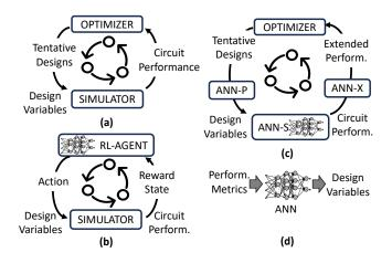
Fig. 2. Circuit design methods. (a) Simulation-based approach. (b) ANNdriven simulation-based approach. (c) RL approach. (d) Approach in this work.
