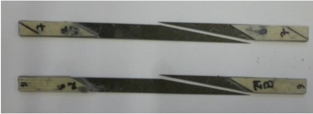
Figure 8. Premature failures in off-axis samples with oblique tabs.
