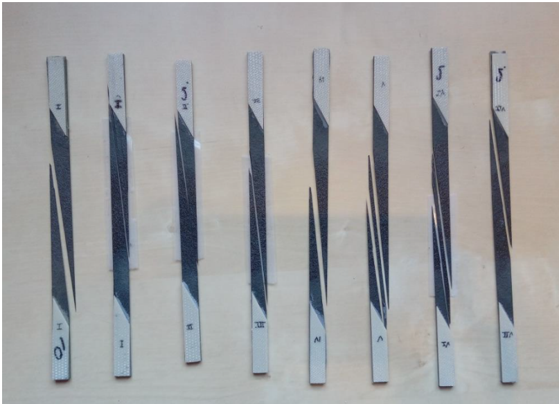
Figure 12.- View of the failure specimens for fibre orientation angle 5°.
