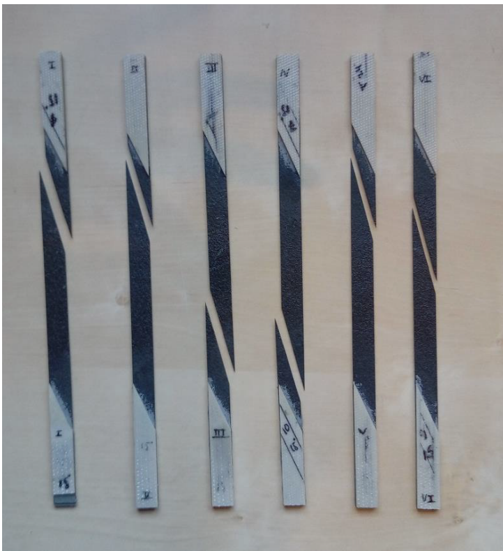
Figure 14.- View of the failure specimens for fibre orientation angle 15^\circ .
