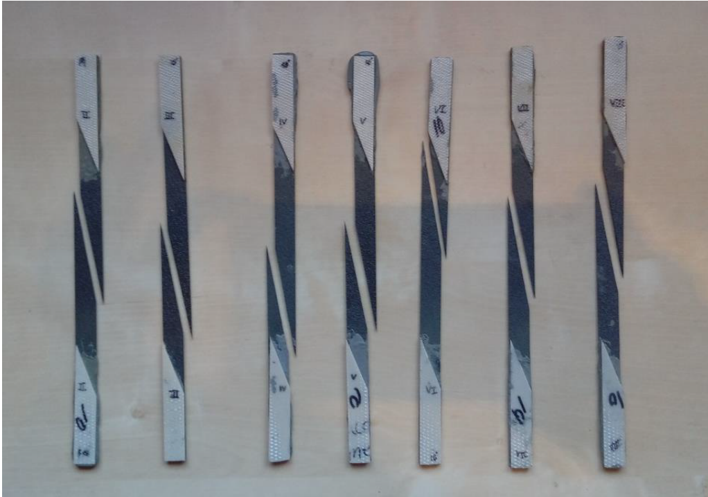
Figure 13.- View of the failure specimens for fibre orientation angle 10^\circ .
