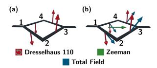
FIG. 1. (a) Square circuit subject to D110 SOC. The arrows represent the SOC field experienced by CCW propagating spin carriers. The field lies in the vertical direction, pointing up or down depending on the carriers'  $p_y$  momentum at each circuit's section. For CW propagating carriers, the SOC field inverts its sign due to time-reversal symmetry. (b) The introduction of a Zeeman field activates discontinuities in the effective-field direction localized at vertices 2 and 4.
