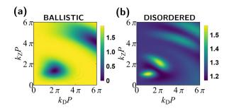
FIG. 2. Tight-binding simulation of the quantum conductance (in units of  $e^2/h$ ) for 1D square loops corresponding to (a) a symmetric circuit in the ballistic regime and (b) a disordered circuit.
